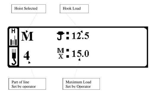
The top row of the display window shows Selected Hoist and Hook Load. The bottom row shows the Parts of line selected and the maximum Load set by the operator.
