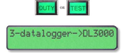
Press the ACKN button, all the data recorded by the 650v3 will be transferred to the external data transfer module.
