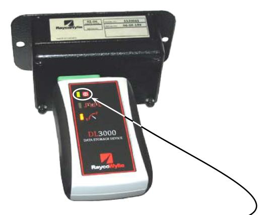
• When the transfer module is connected, verify that the power on light is **green**.
