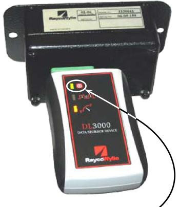
• When the transfer module is connected, verify that the power on light is **green**.
